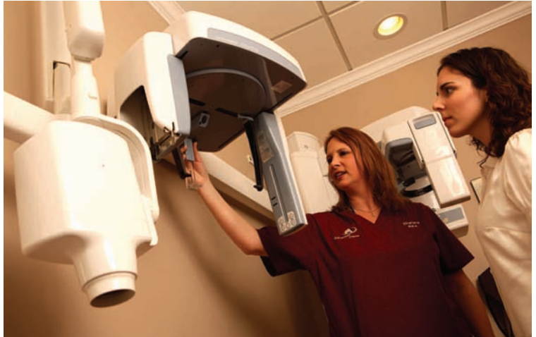
Charlene (left) takes a cephalometric X-ray on an orthodontic patient using the Instrumentarium Orthoceph OC 200D.
